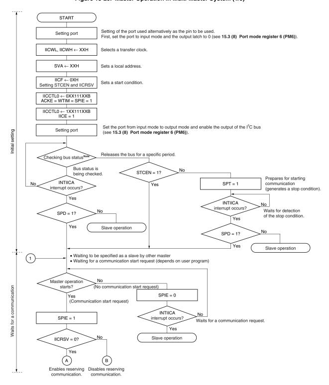
**Note** Confirm that the bus is released (CLD bit = 1, DAD bit = 1) for a specific period (for example, for a period of one frame). If the SDA0 pin is constantly at low level, decide whether to release the I<sup>2</sup>C bus (SCL0 and SDA0 pins = high level) in conformance with the specifications of the product that is communicating.
