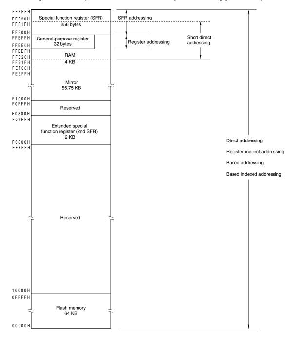
Figure 3-5. Correspondence Between Data Memory and Addressing (μPD78F1016)
