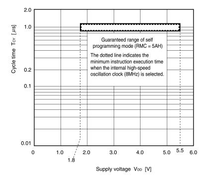
**Remark** The self programming function cannot be used when the CPU operates with the subsystem clock.
