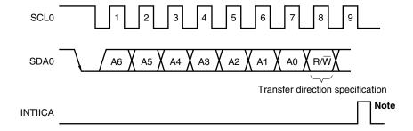
**Note** INTIICA is not issued if data other than a local address or extension code is received during slave device operation.
