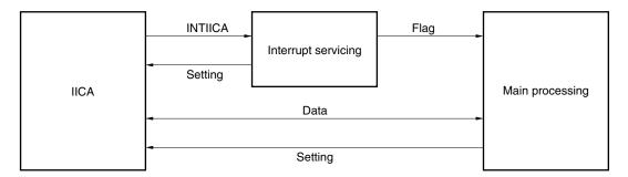
Therefore, data communication processing is performed by preparing the following three flags and passing them to the main processing instead of INTIICA.
