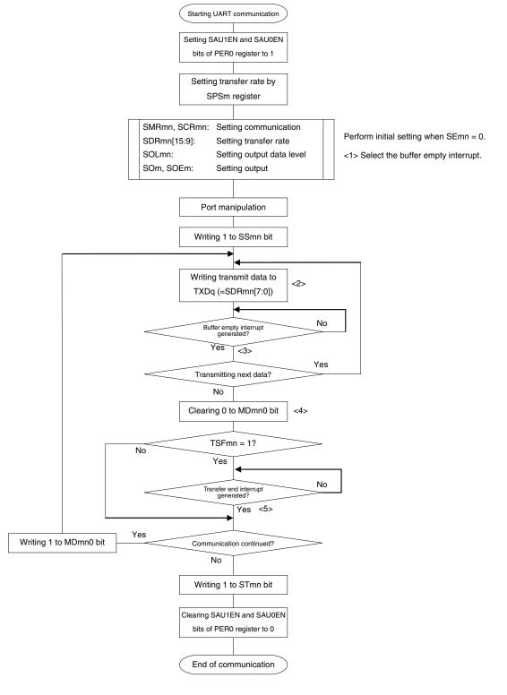
Figure 14-75. Flowchart of UART Transmission (in Continuous Transmission Mode)
