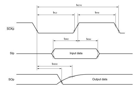
CSI mode serial transfer timing (communication at different potential) (When DAPmn = 0 and CKPmn = 1, or DAPmn = 1 and CKPmn = 0.)
