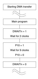
Caution When DMA transfer is held pending while using both DMA channels, be sure to held the DMA transfer pending for both channels (by setting DWAIT0 and DWAIT1 to 1). If the DMA transfer of one channel is executed while that of the other channel is held pending, DMA transfer might not be held pending for the latter channel.
