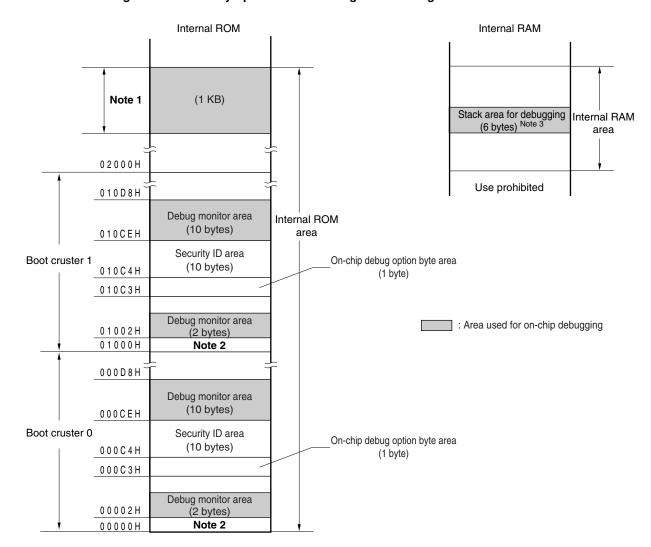
Figure 26-2. Memory Spaces Where Debug Monitor Programs Are Allocated
