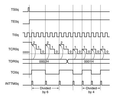
Figure 6-46. Example of Set Contents of Registers When Frequency Divider Is Used
