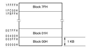
Correspondence between the address values and block numbers in the flash memory are shown below.
