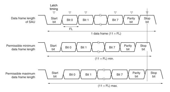
As shown in Figure 14-87, the timing of latching receive data is determined by the division ratio set by bits 15 to 9 of the serial data register mn (SDRmn) after the start bit is detected. If the last data (stop bit) is received before this latch timing, the data can be correctly received.
