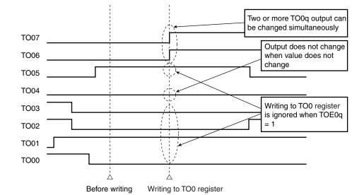
Figure 6-32. TO0q Pin Statuses by Collective Manipulation of TO0q Bits
