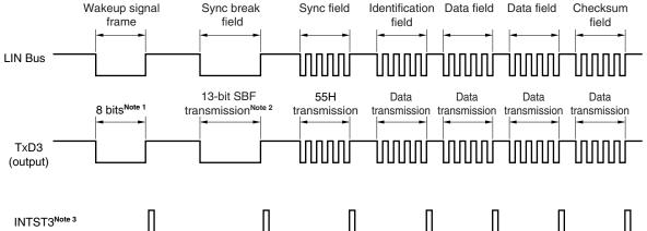
Figure 14-82. Transmission Operation of LIN
