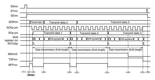
**Note** When transmit data is written to the SDRmn register while BFFmn = 1, the transmit data is overwritten.
