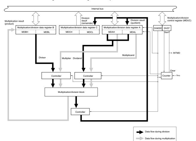
Figure 16-1. Block Diagram of Multiplier/Divider
