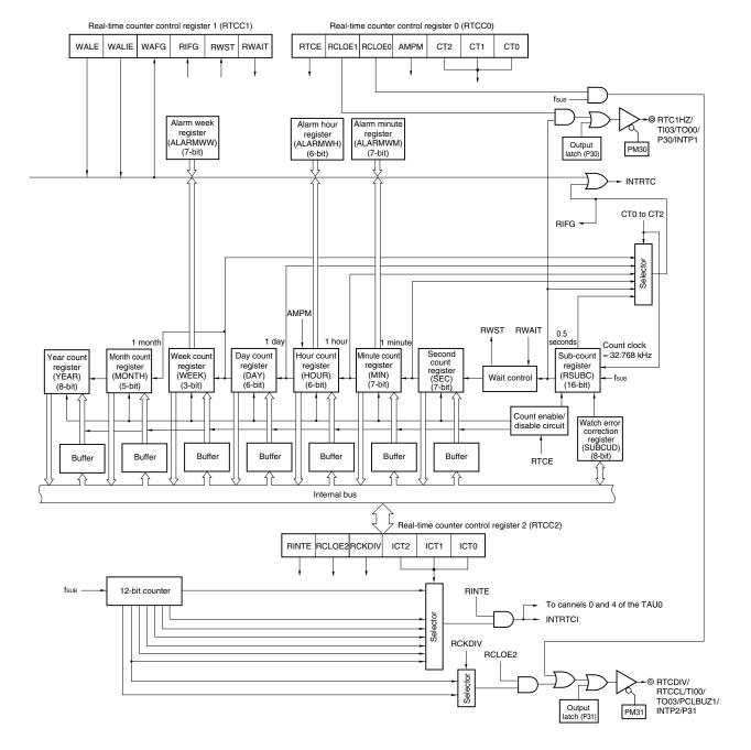
Figure 7-1. Block Diagram of Real-Time Counter
