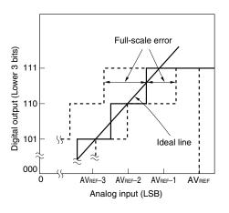
Figure 10-25. Differential Linearity Error
