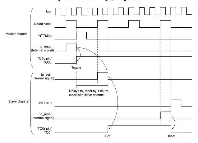
Remarks 1. to\_reset: TO0q pin reset/toggle signal
