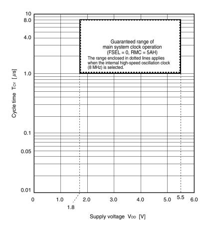
**Remarks 1.** FSEL: Bit 0 of the operation speed mode control register (OSMC)
