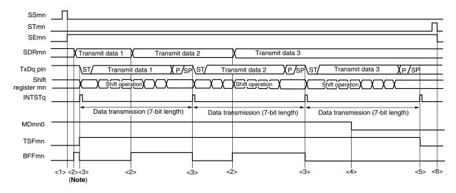
Note When transmit data is written to the SDRmn register while BFFmn = 1, the transmit data is overwritten.
