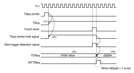
Caution In the first cycle operation of count clock after writing TSpq, an error at a maximum of one clock is generated since count start delays until count clock has been generated. When the information on count start timing is necessary, an interrupt can be generated at count start by setting MDpq0 = 1.
