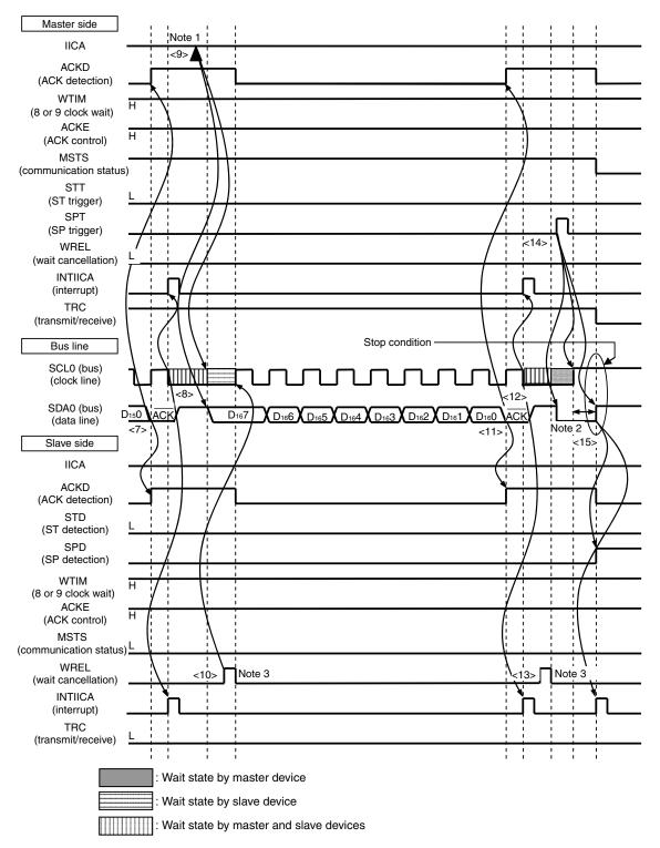
Notes 1. Write data to IICA, not setting the WREL bit, in order to cancel a wait state during master transmission.
