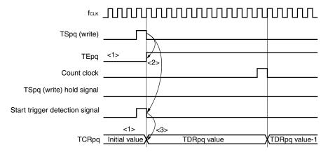
Figure 6-12. Start Timing (In Event Counter Mode)
