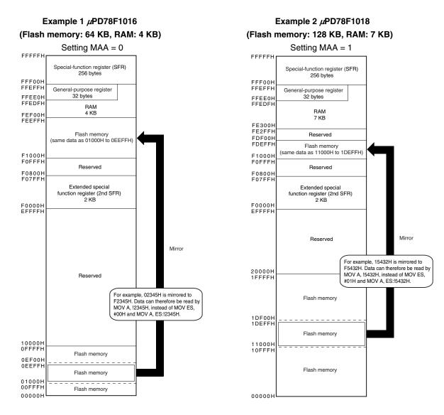
Remark MAA: Bit 0 of the processor mode control register (PMC).
