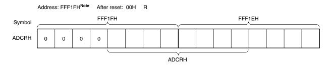
**Note** If address FFF1FH is read, the data of ADCRH (lower four bits of FFF1FH and higher four bits of FFF1EH) will be read.
