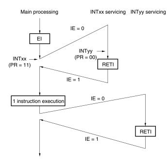
Interrupts are not enabled during servicing of interrupt INTxx (EI instruction is not issued), therefore, interrupt request INTyy is not acknowledged and multiple interrupt servicing does not take place. The INTyy interrupt request is held pending, and is acknowledged following execution of one main processing instruction.
