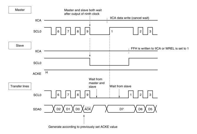
Remark ACKE: Bit 2 of IICA control register 0 (IICCTL0)
