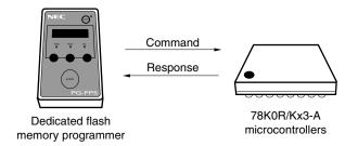
The flash memory control commands of the 78K0R/Kx3-A microcontrollers are listed in the table below. All these commands are issued from the programmer, and the 78K0R/Kx3-A microcontrollers perform processing corresponding to the respective commands.
