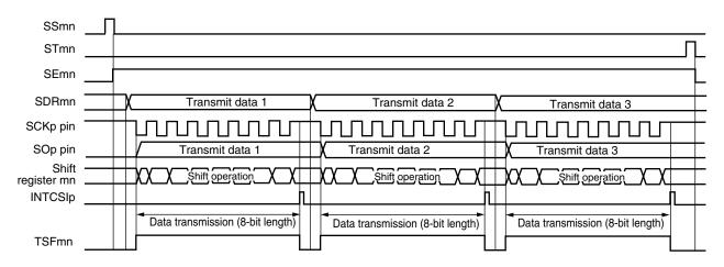
Starting CSI communication Setting SAU1EN and SAU0EN bits of PER0 register to 1 Setting transfer rate by SPSm register SMRmn, SCRmn: Setting communication SDRmn[15:9]: Setting transfer rate Perform initial setting when SEmn = 0. SOm, SOEm: Setting output Port manipulation Writing 1 to SSmn bit Writing transmit data to SIOp (=SDRmn[7:0]) No Transfer end interrupt generated? No Transmission completed? Writing 1 to STmn bit Clearing SAU1EN and SAU0EN bits of PER0 register to 0 End of communication
