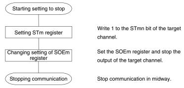
Remarks 1. Even after communication is stopped, the pin level is retained. To resume the operation, re-set the SOm register (see Figure 14-41 Procedure for Resuming Master Transmission/Reception).
