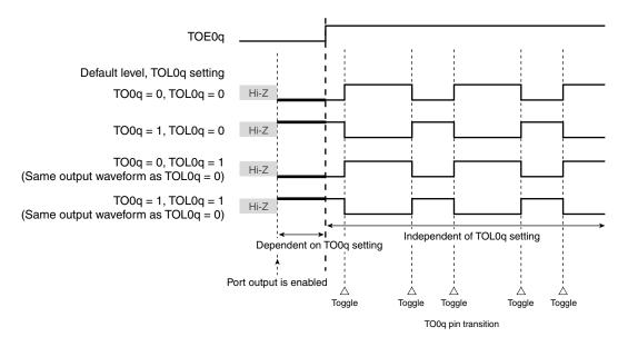
Figure 6-27. TO0g Pin Output Status at Toggle Output (TOM0g = 0)
