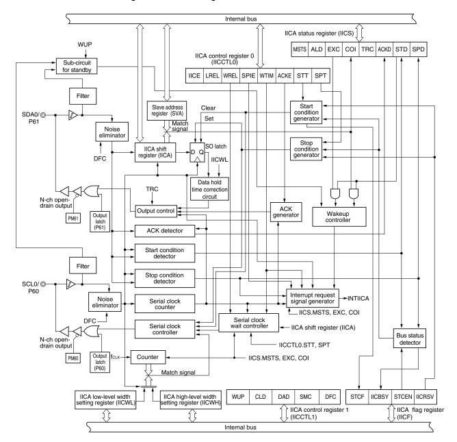
Figure 15-1. Block Diagram of Serial Interface IICA
