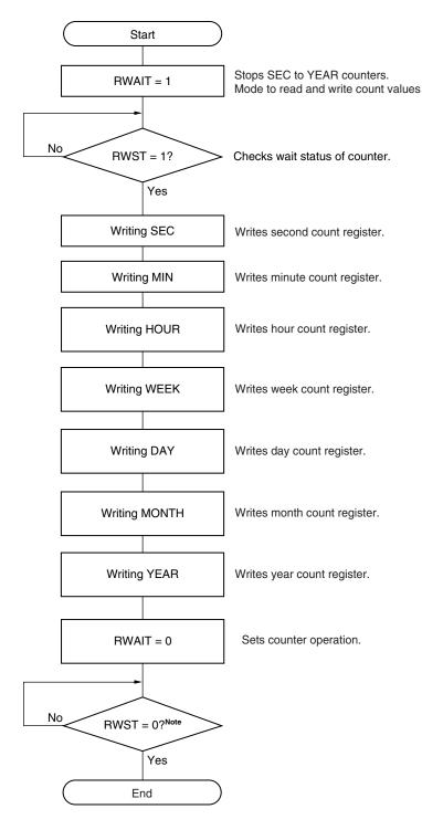
Figure 7-22. Procedure for Writing Real-Time Counter
