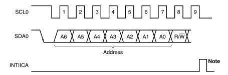
**Note** INTIICA is not issued if data other than a local address or extension code is received during slave device operation.
