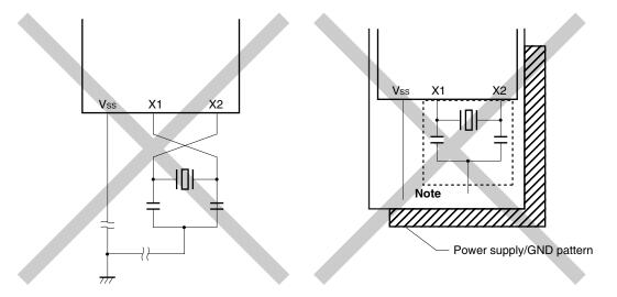
**Note** Do not place a power supply/GND pattern underneath the wiring section (in broken lines above) of the X1 and X2 pins and resonator in the multilayer board and double-sided board.
