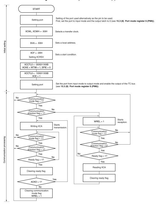
Figure 15-30. Slave Operation Flowchart (1)
