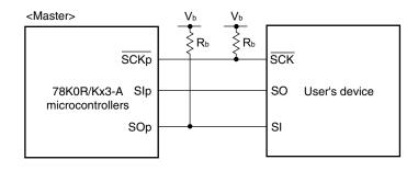
Caution Select the TTL input buffer for SIp and the N-ch open drain output (VDD tolerance) mode for SOp and SCKp by using the PIMg and POMx registers.
