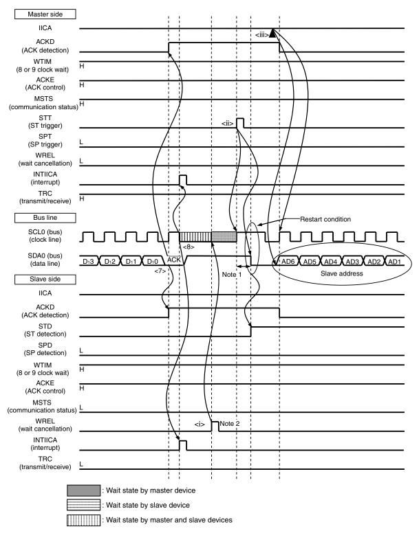
**Notes 1.** Make sure that the time between the rise of the SCL0 pin signal and the generation of the start condition after a restart condition has been issued is at least 4.7  $\mu$ s when specifying standard mode and at least 0.6  $\mu$ s when specifying fast mode.
