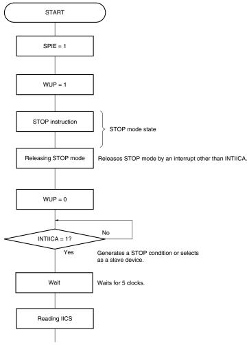
Executes processing corresponding to the operation to be executed after checking the operation state of serial interface IICA.
