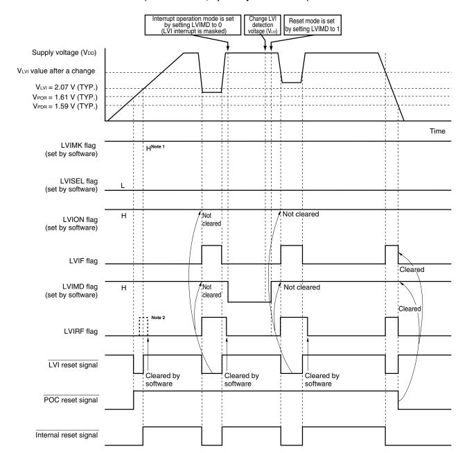
Figure 22-6. Timing of Low-Voltage Detector Internal Reset Signal Generation (Bit: LVISEL = 0, Option Byte: LVIOFF = 0)
