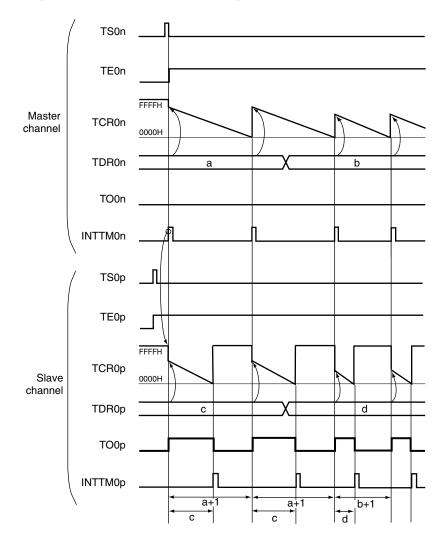
Figure 6-57. Example of Basic Timing of Operation as PWM Function
