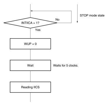
Executes processing corresponding to the operation to be executed after checking the operation state of serial interface IICA.
