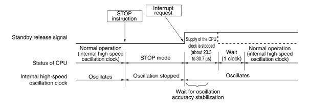
**Remark** The broken lines indicate the case when the interrupt request that has released the standby mode is acknowledged.
