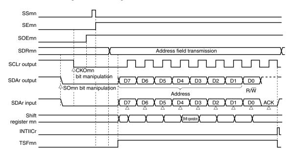
Starting IIC communication SMRmn, SCRmn: Setting communication SPSm, SDRmn[15:9]: Setting transfer rate Writing 0 to SOmn bit Perform initial setting when SEmn = 0. Writing 0 to CKOmn bit Writing 1 to SOEmn bit Writing 1 to SSmn bit Writing address and R/W data to SIOr (SDRmn[7:0]) Transfer end interrupt generated? No Yes Yes Parity error (ACK error) flag PEFmn = 1 ? No ACK reception error Address field transmission completed To data transmission flow and data reception flow
