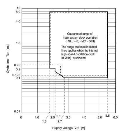
Remark FSEL: Bit 0 of the operation speed mode control register (OSMC)
