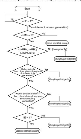
Figure 18-7. Interrupt Request Acknowledgment Processing Algorithm
