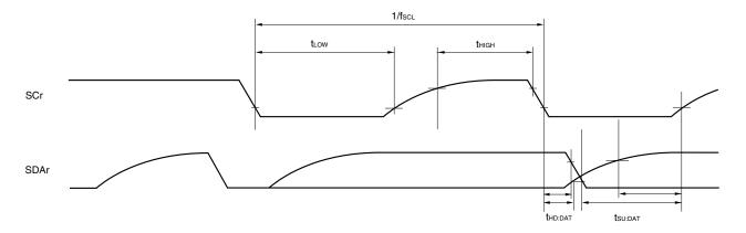
Caution Select the TTL input buffer and the N-ch open drain output (VDD tolerance) mode for SDAr and the N-ch open drain output (VDD tolerance) mode for SCLr by using the PIMg and POMx registers.
