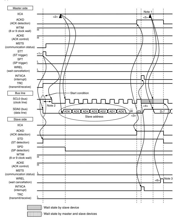
**Notes 1.** Write data to IICA, not setting the WREL bit, in order to cancel a wait state during master transmission.
