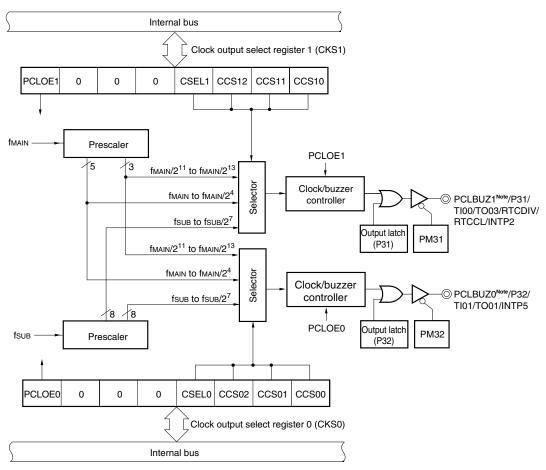
Note The PCLBUZ0 and PCLBUZ1 pins can output a clock of up to 10 MHz at 2.7 V ≤ V<sub>DD</sub>. Setting a clock exceeding 5 MHz at V<sub>DD</sub> < 2.7 V is prohibited.
