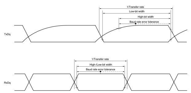
Caution Select the TTL input buffer for RxDq and the N-ch open drain output (VDD tolerance) mode for TxDq by using the PIMg and POMx registers.
