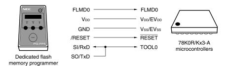
When using the FlashPro5 as the dedicated flash memory programmer, the FlashPro5 generates the following signals for the 78K0R/Kx3-A microcontrollers. For details, refer to the user's manual for the FlashPro5.
