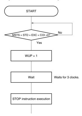
Figure 15-22. Flow When Setting WUP = 1
