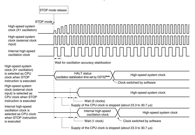
**Note** When the oscillation stabilization time set by OSTS is equal to or shorter than 61  $\mu$ s, the HALT status is retained to a maximum of "61 $\mu$ s + wait time."
