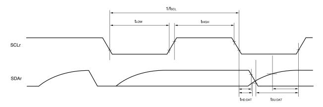
$\label{eq:Remarks 1.} $$R_b[\Omega]$: Communication line (SDAr) pull-up resistance, $$C_b[F]$: Communication line (SCLr, SDAr) load capacitance$
