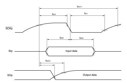
Caution Select the TTL input buffer for SIp and the N-ch open drain output (VDD tolerance) mode for SOp and SCKp by using the PIMg and POMx registers.
