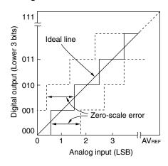
Figure 10-24. Integral Linearity Error
