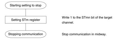
**Remarks 1.** Even after communication is stopped, the pin level is retained. To resume the operation, reset the SOm register (see **Figure 14-35 Procedure for Resuming Master Reception**).
