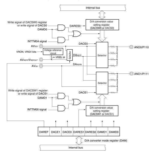
Figure 11-1. Block Diagram of D/A Converter
