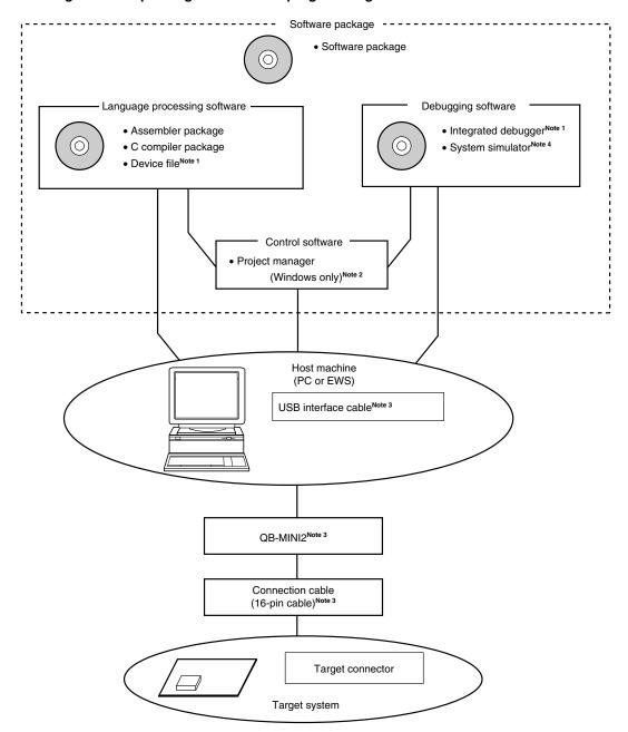
**Notes 1.** Download the device file for 78K0R/Kx3-A microcontrollers (DF781018) and the integrated debugger ID78K0R-QB from the download site for development tools (http://www2.renesas.com/micro/en/ods/).
