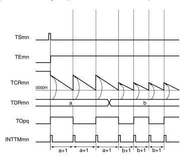
**Remark** mn = 00 to 07, 10 to 13: Unit number + Channel number pq = 00 to 07: Unit number + Channel number (only for channels provided with timer I/O pins)
