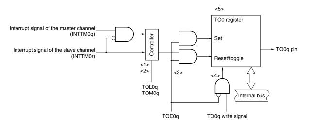
The following describes the TO0q pin output circuit.
