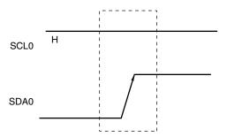
A stop condition is generated when bit 0 (SPT) of IICA control register 0 (IICCTL0) is set to 1. When the stop condition is detected, bit 0 (SPD) of the IICA status register (IICS) is set to 1 and INTIICA is generated when bit 4 (SPIE) of IICCTL0 is set to 1.
