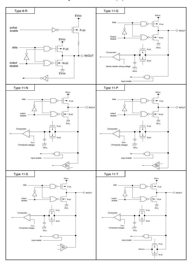
Figure 2-1. Pin I/O Circuit List (3/3)
