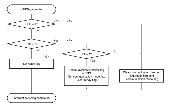
Figure 15-31. Slave Operation Flowchart (2)
