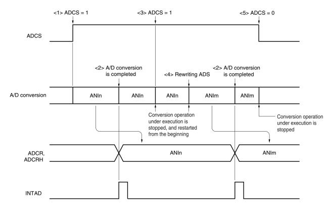
Figure 10-16. Software trigger mode (Continuous conversion mode)
