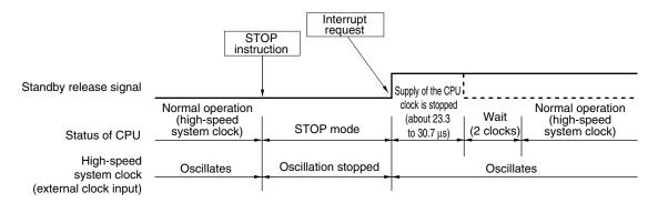
**Remark** The broken lines indicate the case when the interrupt request that has released the standby mode is acknowledged.
