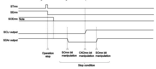
Note During the receive operation, the SOEmn bit is set to 0 before receiving the last data.
