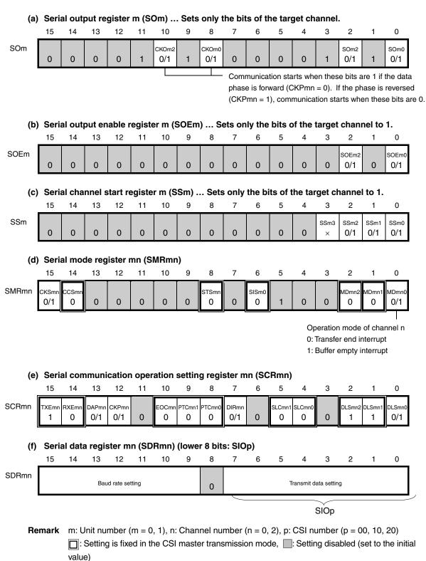
×: Bit that cannot be used in this mode (set to the initial value when not used in any mode)
