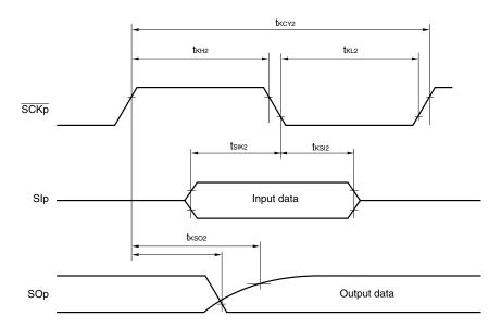
Caution Select the TTL input buffer for SIp and SCKp and the N-ch open drain output (VDD tolerance) mode for SOp by using the PIMg and POMx registers.
