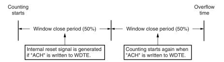
Caution When data is written to WDTE for the first time after reset release, the watchdog timer is cleared in any timing regardless of the window open time, as long as the register is written before the overflow time, and the watchdog timer starts counting again.
