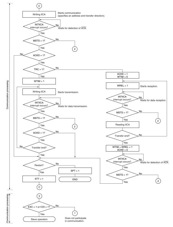
Figure 15-29. Master Operation in Multi-Master System (3/3)
