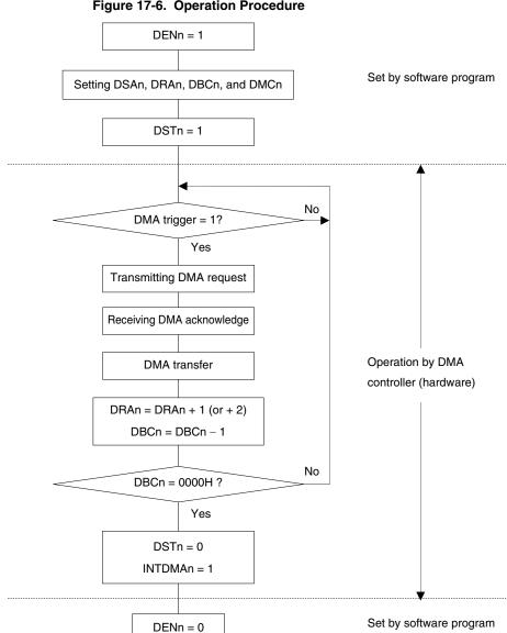
Figure 17-6. Operation Procedure
