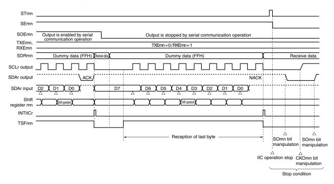
Address field transmission completed Writing 1 to STmn bit Writing 0 to TXEmn bit, and 1 to RXEmn bit Writing 1 to SSmn bit Starting data reception Yes Last byte received? Writing 0 to SOEmn bit No (Stopping output by serial communication operation) Writing dummy data (FFH) to SIOr (SDRmn[7:0]) Transfer end interrupt generated? No Yes Reading SIOr (SDRmn[7:0]) No Data transfer completed? Yes Data reception completed Stop condition generation
