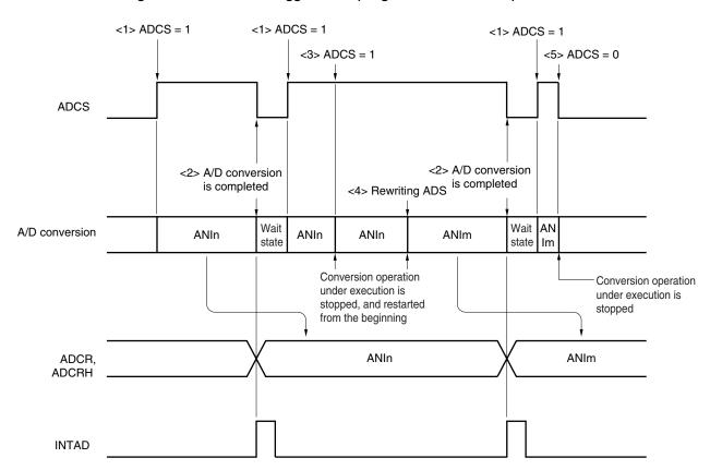
Figure 10-17. Software trigger mode (Single conversion mode)
