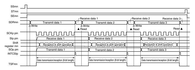
Figure 14-65. Flowchart of Slave Transmission/Reception (in Single-Transmission/Reception Mode)
