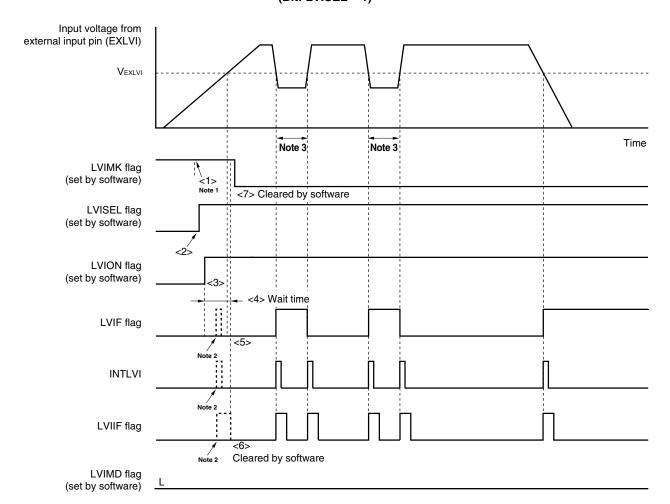
Figure 22-10. Timing of Low-Voltage Detector Interrupt Signal Generation
