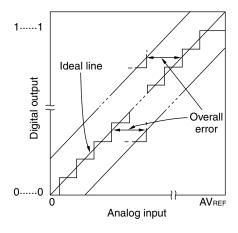
Figure 10-21. Quantization Error
