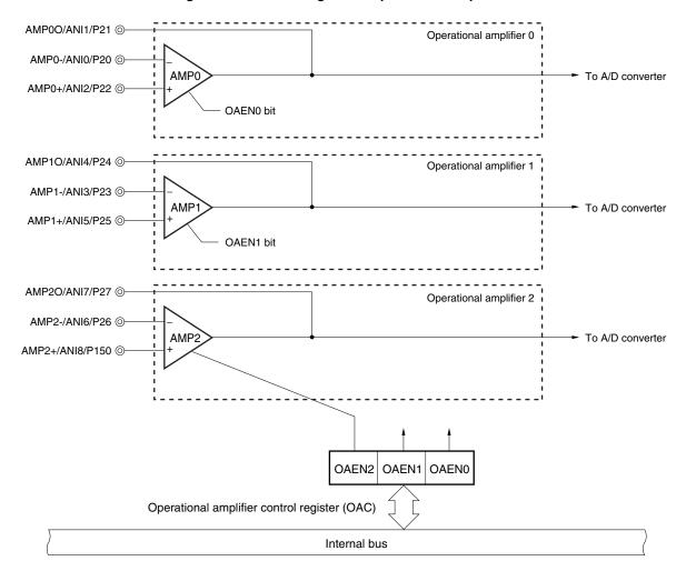
Figure 12-1. Block Diagram of Operational Amplifiers
