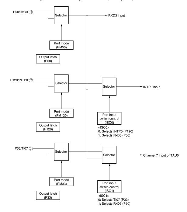
Figure 14-85. Port Configuration for Manipulating Reception of LIN
