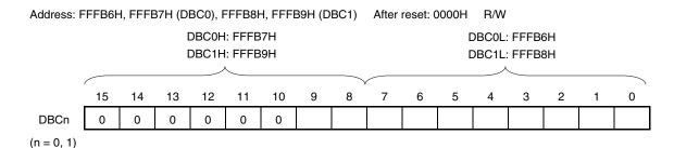
DBCn[9:0] Number of Times of Transfer Remaining Number of Times of Transfer (When DBCn is Written) (When DBCn is Read) 000H 1024 Completion of transfer or waiting for 1024 times of DMA transfer 001H 1 Waiting for remaining one time of DMA transfer 002H 2 Waiting for remaining two times of DMA transfer 003H Waiting for remaining three times of DMA transfer 3 3FEH 1022 Waiting for remaining 1022 times of DMA transfer 3FFH 1023 Waiting for remaining 1023 times of DMA transfer
