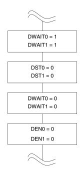
Caution In example 3, the system is not required to wait two clock cycles after the DWAITn bit is set to 1. In addition, the system does not have to wait two clock cycles after clearing the DSTn bit to 0, because more than two clock cycles elapse from when the DSTn bit is cleared to 0 to when the DENn bit is cleared to 0.
