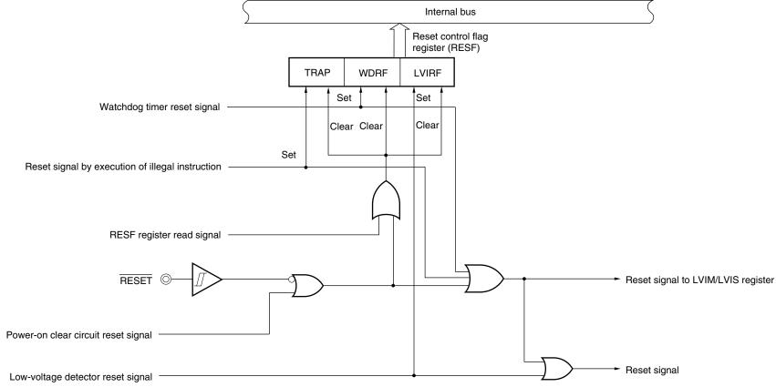
Caution An LVI circuit internal reset does not reset the LVI circuit.
