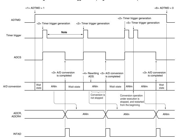
Figure 10-19. Timer trigger mode (Single conversion mode)
