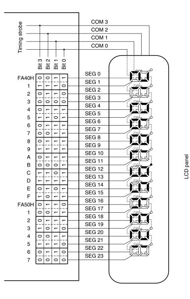
Figure 18-28. Example of Connecting Four-Time-Slice LCD Panel
