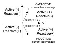
Figure 22-51. Signs for Active Power and Reactive Power
