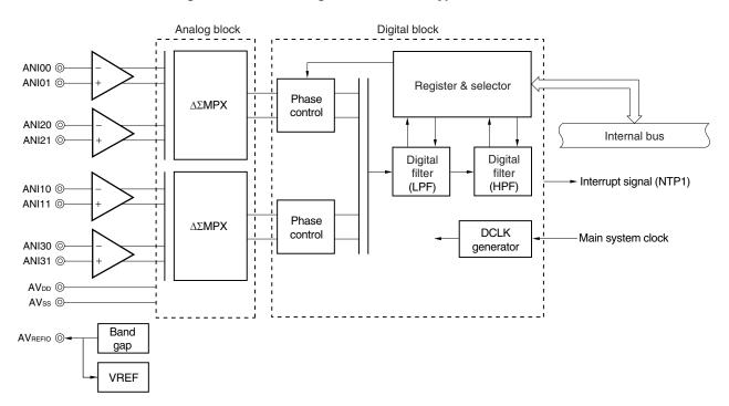
Figure 13-1. Block Diagram of 24-bit ΔΣ-Type A/D Converter
