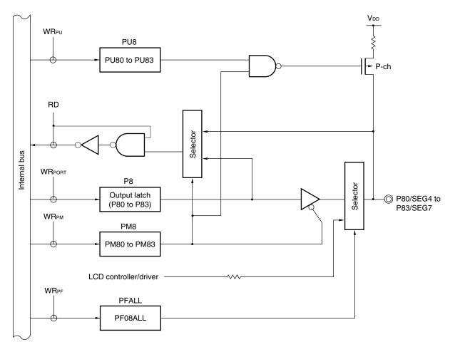
Figure 4-11. Block Diagram of P80 to P83
