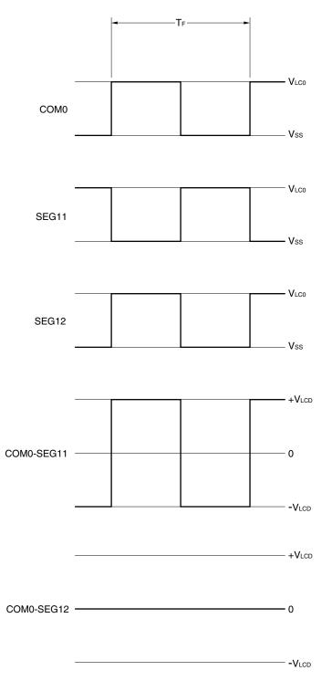
Figure 18-19. Static LCD Drive Waveform Examples
