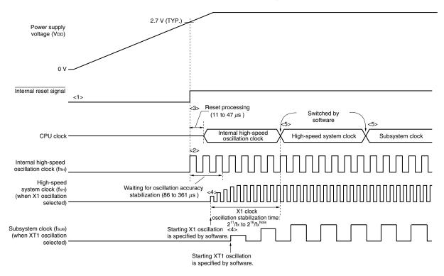
Figure 5-15. Clock Generator Operation When Power Supply Voltage Is Turned On (When 2.7 V/1.59 V POC Mode Is Set (Option Byte: POCMODE = 1))
