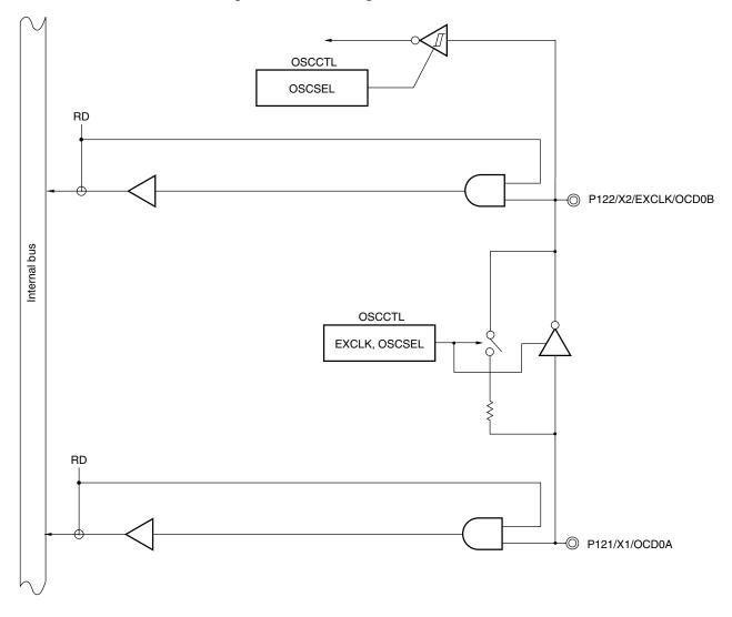
Figure 4-18. Block Diagram of P121 and P122
