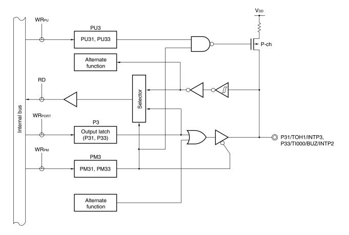
Figure 4-7. Block Diagram of P31, P33
