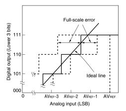
Figure 12-19. Differential Linearity Error
