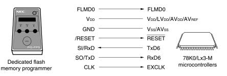
The dedicated flash memory programmer generates the following signals for the 78K0/Lx3-M microcontrollers. For details, refer to the user's manual for the PG-FP5 or FL-PR5.
