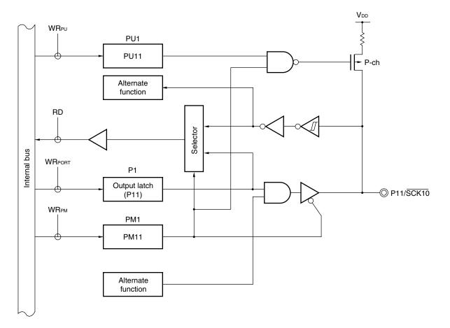
Figure 4-1. Block Diagram of P11
