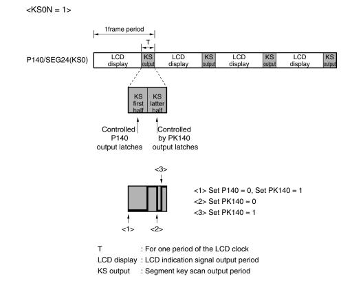
RemarkDuring the segment key scan output period, COM will not be displayed when output.See Figure 18-15 and Figure 18-16 for waveform details.
