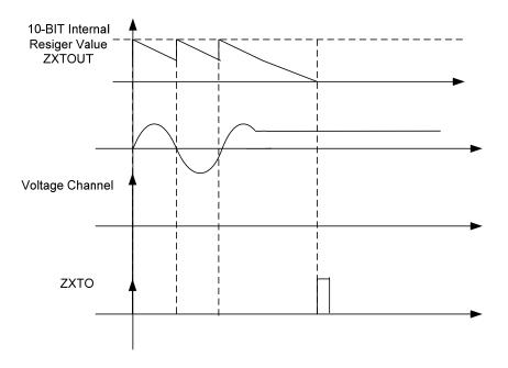
Figure 23-18. Internal Counter of ZXOUTn Register
