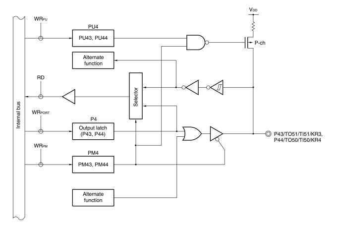
Figure 4-10. Block Diagram of P43 and P44
