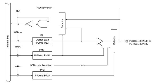
Figure 4-4. Block Diagram of P20 to P27 (78K0/LG3-M)
