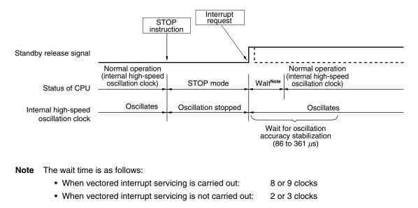
**Remark** The broken lines indicate the case when the interrupt request that has released the standby mode is acknowledged.
