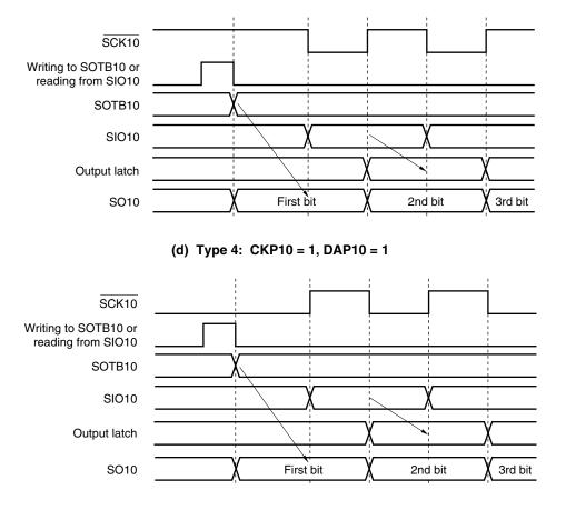
Figure 16-8. Output Operation of First Bit (2/2)
