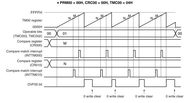
Figure 6-25. Timing Example of Free-Running Timer Mode (CR000: Compare Register, CR010: Compare Register)
