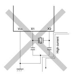
Figure 5-13. Examples of Incorrect Resonator Connection (2/2)
