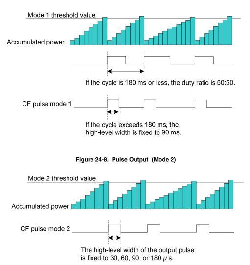
Cautions 1. In mode 1, if the cycle exceeds 180 ms, the high-level width is fixed to 90 ms.
