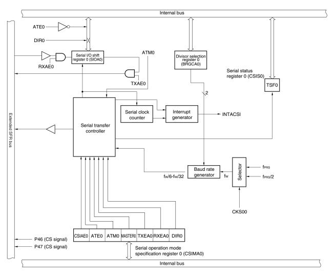
Figure 17-1. Block Diagram of Extended SFR Interface
