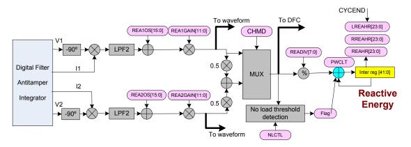
The reactive energy accumulation method can be selected by specifying values for the SAVARM and ABSVARM bits in the PWCTL2 register. For details about the accumulation method, see **22.4.5 (2) (c) Reactive energy accumulation modes**.
