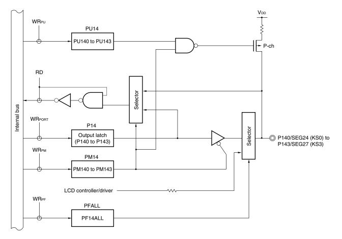
Figure 4-21. Block Diagram of P140 to P143
