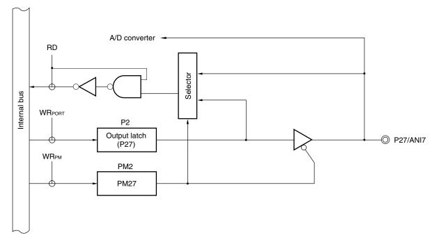
Figure 4-5. Block Diagram of P27 (78K0/LE3-M)
