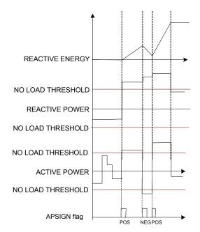
This mode also applies to CF pulse output. The default setting for this mode is off. Detection of transitions in the direction of power flow and detection of the no-load threshold are enabled in this mode.
