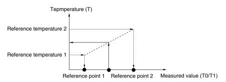
RTC correction is performed by calculating the correction value using the temperature measurement results. For the oscillation frequency, RTC correction can correct the frequency error in the range from -189 to +189 ppm.
