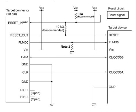
Figure 31-1. Connection Example of QB-MINI2 and 78K0/Lx3-M microcontrollers
