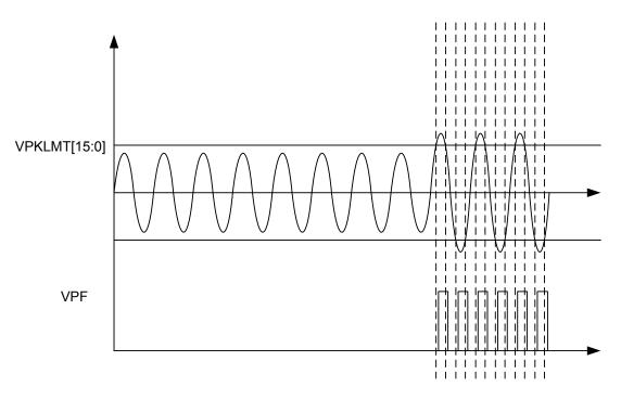
Figure 23-24. Peak Detection Timing
