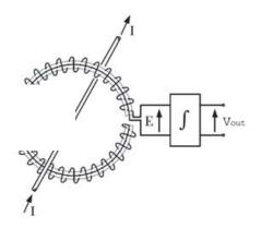
If using a Rogowski coil as a current sensor, the input current signal is a di/dt signal, and, because the current signal must be restored before the power can be calculated, an integrator is included.
