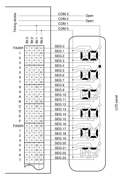
Figure 18-21. Example of Connecting Two-Time-Slice LCD Panel
