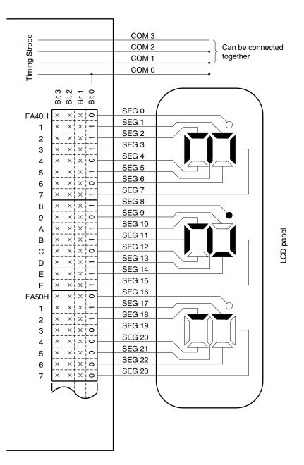
Figure 18-18. Example of Connecting Static LCD Panel
