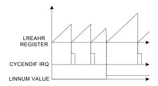
The CYCDIS bit in the PWCTL1 register can disable CYCEND detection. If the CYCDIS bit is set to 1, the CYCEND interrupt will not occur when the number of half-line cycles reaches the value specified for the LINNUM register. Also, if the CYCDIS bit is set to 1, the LREAHR register and inner accumulation register will not reset to 0 when a new half-line cycle is written to the LINNUM register.
