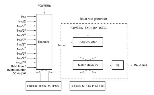
Figure 15-24. Configuration of Baud Rate Generator
