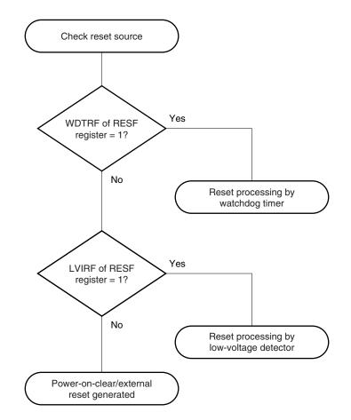
Figure 27-3. Example of Software Processing After Reset Release (2/2)
