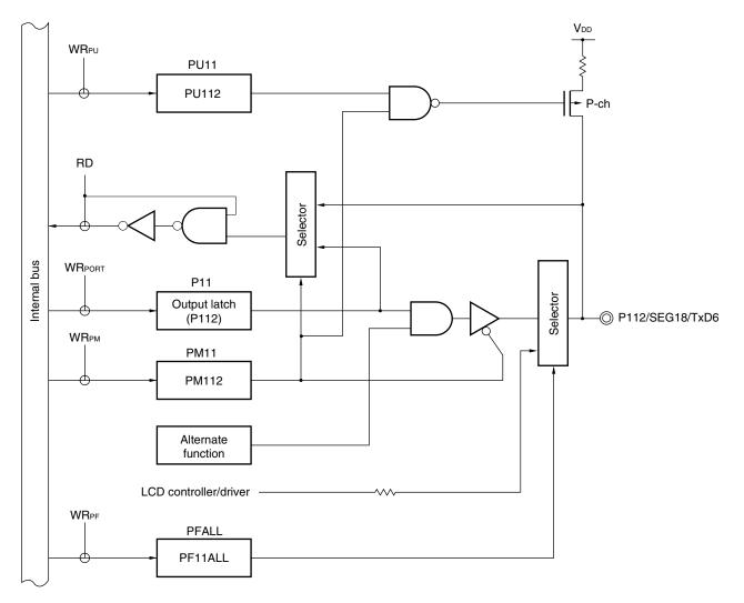
Figure 4-15. Block Diagram of P112
