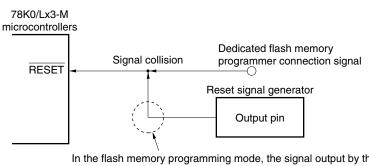
Figure 30-9. Signal Collision (RESET Pin)
