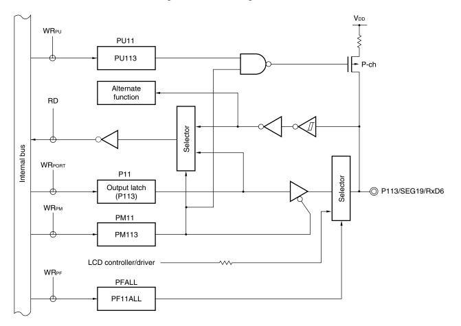
Figure 4-16. Block Diagram of P113
