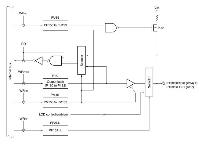
Figure 4-22. Block Diagram of P150 to P153
