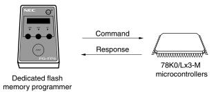
The flash memory control commands of the 78K0/Lx3-M microcontrollers are listed in the table below. All these commands are issued from the programmer and the 78K0/Lx3-M microcontrollers perform processing corresponding to the respective commands.
