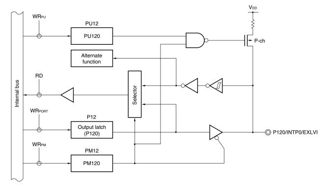
Figure 4-17. Block Diagram of P120
