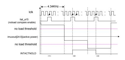
Figure 22-76. INTACTNOLD Interrupt (Active Power)
