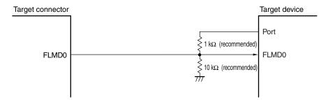
Caution When using the port that controls the FLMD0 pin, make sure that it satisfies the values of the highlevel output current and FLMD0 supply voltage (minimum value: 0.8Vpb) stated in CHAPTER 33 ELECTRICAL SPECIFICATIONS.
