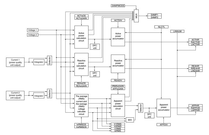
Figure 22-1. Block Diagram of Power Calculation Circuit
