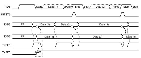
Figure 15-17. Timing of Starting Continuous Transmission
