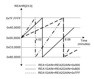
Note that, if an overflow occurs while the power or energy flow is positive, the energy register contents invert to the maximum negative value (0x800000) and then continuously increase in value. Conversely, if the power is negative, after an underflow, the energy register contents switch to the maximum positive value (0x7FFFF) and then continuously decrease in value.
