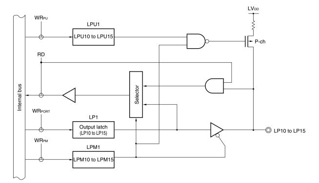
Figure 4-25. Block Diagram of LP10 to LP15
