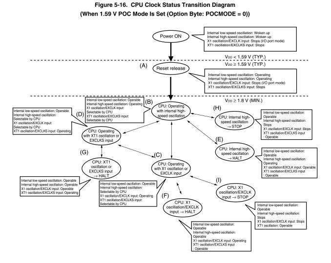
**Remark** In the 2.7 V/1.59 V POC mode (option byte: POCMODE = 1), the CPU clock status changes to (A) in the above figure when the supply voltage exceeds 2.7 V (TYP.), and to (B) after reset processing (11 to 47  $\mu$ s (TYP.)).
