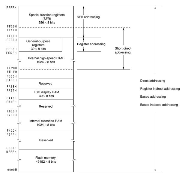
Figure 3-7. Correspondence Between Data Memory and Addressing (µPD78F8054)
