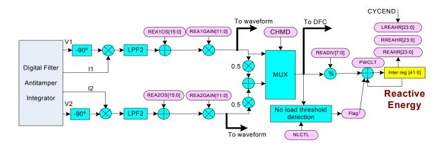
• If CHMD = 0 (the single-phase two-wire mode): reactive power = V1\_ phase-shifted × I1
