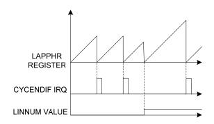
The CYCDIS bit in the PWCTL1 register can disable CYCEND detection. If the CYCDIS bit is set to 1, the CYCEND interrupt will not occur when the number of half-line cycles reaches the value specified for the LINNUM register. Also, if the CYCDIS bit is set to 1, the LAPPHR register and inner accumulation register will not reset to 0 when a new half-line cycle is written to the LINNUM register.
