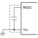
Caution Keep the wiring length as short as possible in the area enclosed by the broken lines in the above figures.
