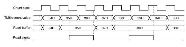
Figure 7-19. 8-bit Timer Counter 5n (TM5n) Read Timing
