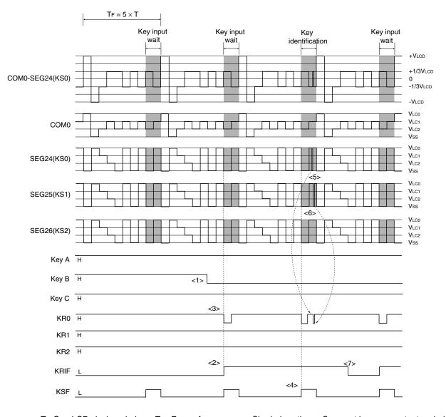
Figure 18-33. Example of Segment Key Scan Operation Timing (Four-Time-Slice (1/3 Bias Method))
