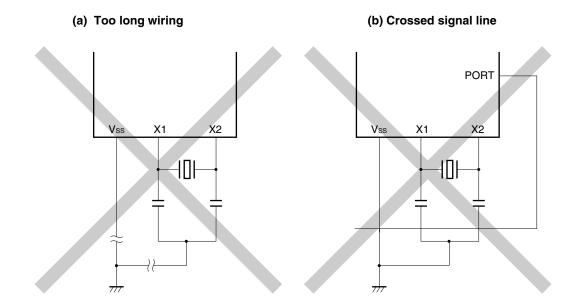
Figure 5-13. Examples of Incorrect Resonator Connection (1/2)
