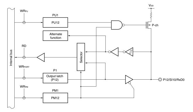
Figure 4-2. Block Diagram of P12
