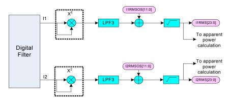
The measured current channel RMS value is stored in the relevant register every 4.34 kHz. Note that, by setting the ZXRMS bit of the NLCTL register to 1, the measurement result can be stored in the register in sync with the line frequency (in sync with the zero-crossing of the input voltage). If the ZXRMS bit is set, the operation is as follows.
