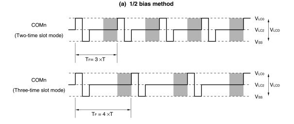
Figure 18-15 Common Signal Waveforms
