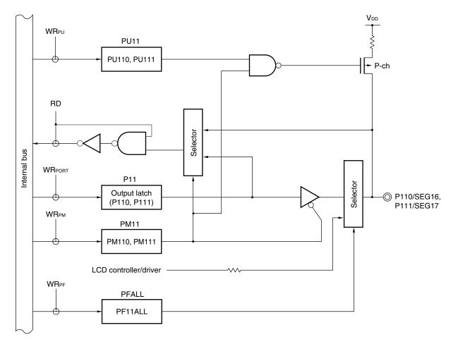
Figure 4-14. Block Diagram of P110 and P111
