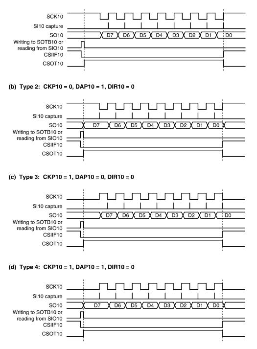
Remark The above figure illustrates a communication operation where data is transmitted with the MSB first.
