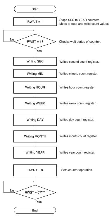
Figure 9-22. Procedure for Writing Real-Time Counter
