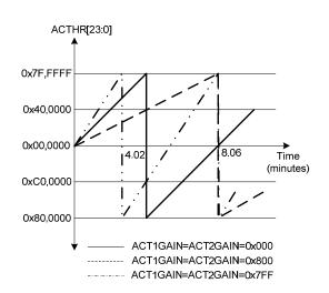
Figure 22-41. Active Energy Accumulation for Full-scale signals
