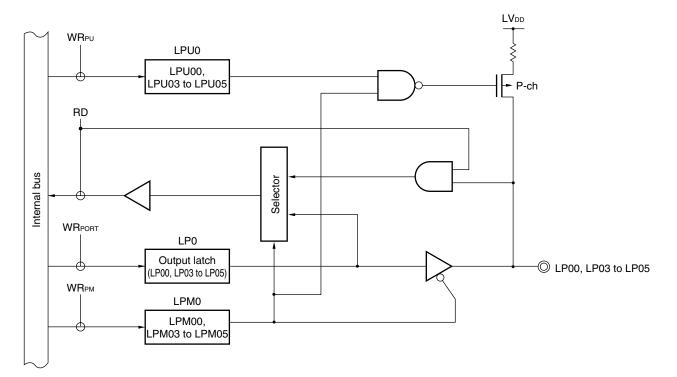
Figure 4-23. Block Diagram of LP00, LP03 to LP05
