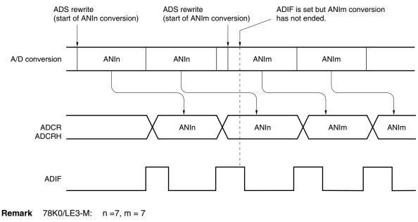
Figure 12-21. Timing of A/D Conversion End Interrupt Request Generation
