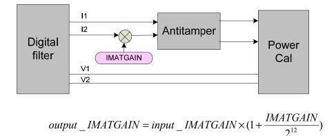
IMATGAIN is a 12-bit signed integer register. The gain resolution for this register is 0.0244% LSB ( $2^{-12} = 0.0244\%$ ).
