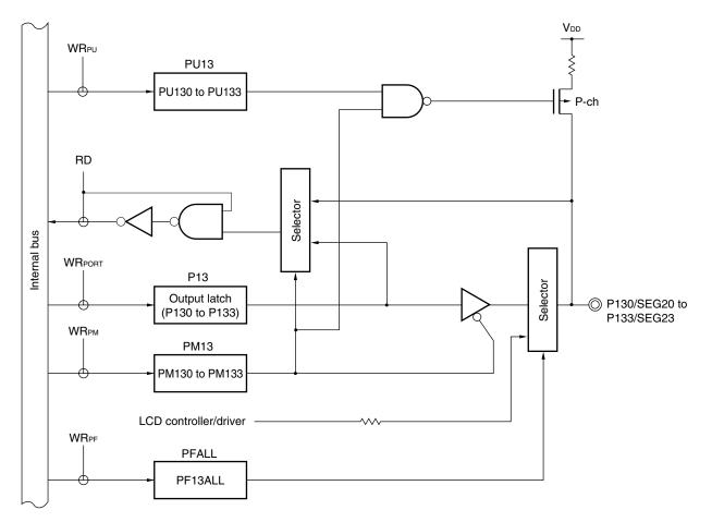
Figure 4-20. Block Diagram of P130 to P133
