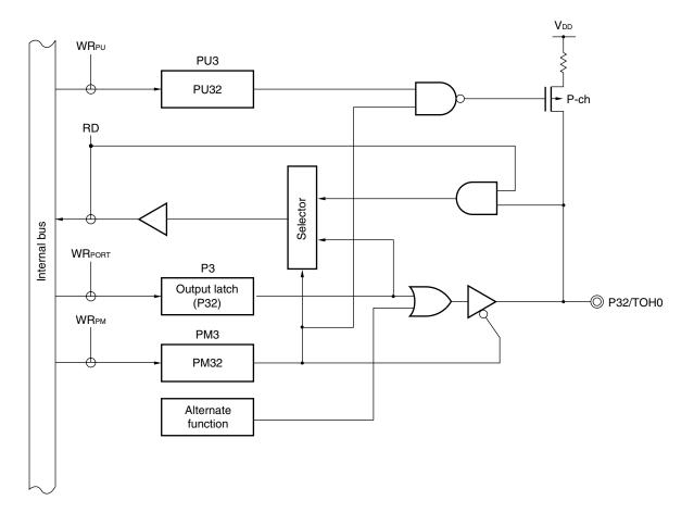
Figure 4-8. Block Diagram of P32
