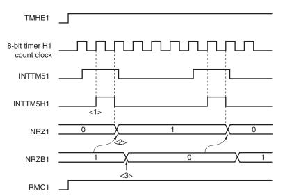
Figure 8-15. Transfer Timing
