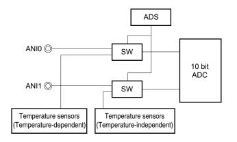
Figure 9-29. Block Diagram of RTC Temperature Correction Circuit
