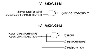
Cautions 1. For the 78K0/LG3-M, the IROUT pin cannot be used at the same time as the P31/TOH1/INTP3 or P13/SO10/TxD0 pin.
