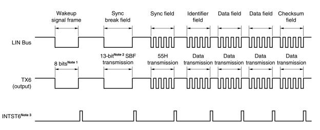
Figure 15-1. LIN Transmission Operation
