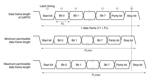
Figure 14-13. Permissible Baud Rate Range During Reception
