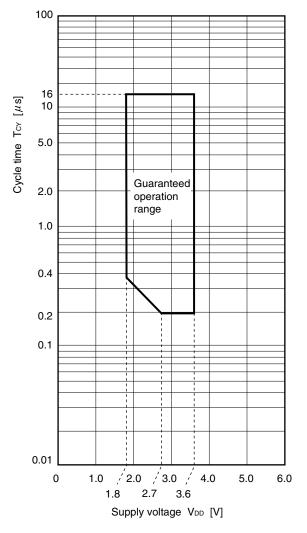
TCY vs. VDD (Main System Clock Operation)
