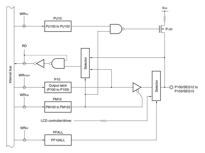
Figure 4-13. Block Diagram of P100 to P103
