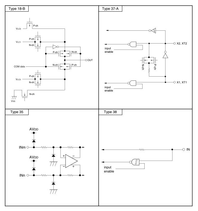
Figure 2-1. Pin I/O Circuit List (3/3)
