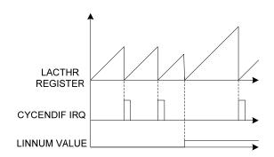
The CYCDIS bit in the PWCTL1 register can disable CYCEND detection. If the CYCDIS bit is set to 1, the CYCEND interrupt will not occur when the number of half-line cycles reaches the value specified for the LINNUM register. Also, if the CYCDIS bit is set to 1, the LACTHR register and inner accumulation register will not reset to 0 when a new half-line cycle is written to the LINNUM register.
