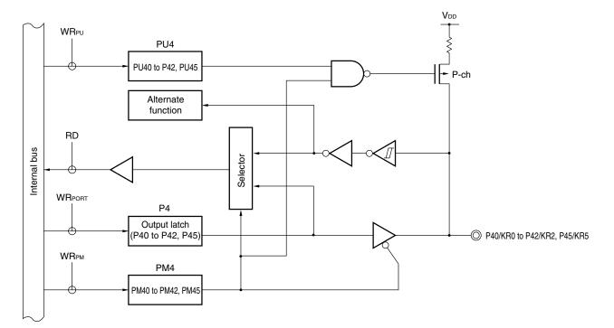
Figure 4-9. Block Diagram of P40 to P42, P45
