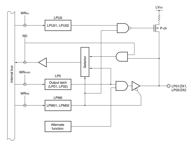
Figure 4-24. Block Diagram of LP01 and LP02
