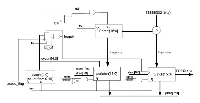
Figure 23-20. Period and Frequency Measurement circuit
