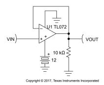
Figure 9-3. Single-Supply Unity Gain Amplifier
