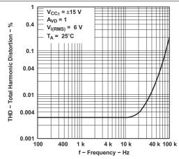
Figure 6-56. Total Harmonic Distortion vs Frequency
