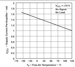
Figure 6-52. Supply Current Per Amplifier vs Free-Air Temperature
