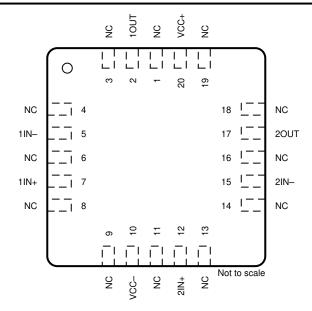
Figure 5-7. TL072 FK Package, 20-Pin LCCC (Top View)
