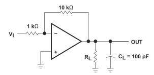
Figure 7-2. Gain-of-10 Inverting Amplifier
