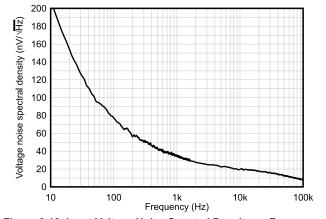
Figure 6-18. Input Voltage Noise Spectral Density vs Frequency
