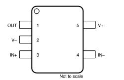
Figure 5-1. TL071H DBV Package, 5-Pin SOT-23 (Top View)
