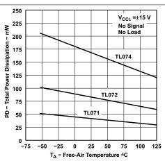
Figure 6-53. Total Power Dissipation vs Free-Air Temperature
