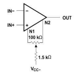
Figure 7-3. Input Offset-Voltage Null Circuit
