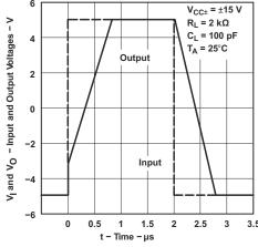
Figure 6-57. Voltage-Follower Large-Signal Pulse Response
