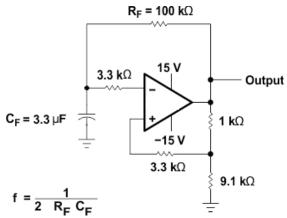
Figure 9-6. 0.5-Hz Square-Wave Oscillator
