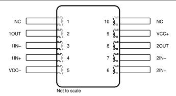
Figure 5-6. TL072x U Package, 10-Pin CFP (Top View)
