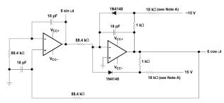
Figure 9-8. 100-kHz Quadrature Oscillator
