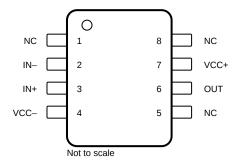
Figure 5-3. TL071H D Package, 8-Pin SOIC (Top View)
