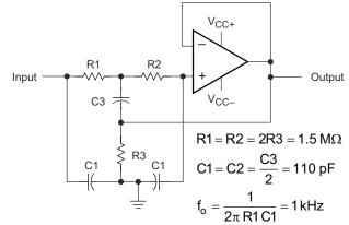
Figure 9-7. High-Q Notch Filter
