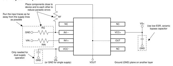
Figure 9-10. Operational Amplifier Board Layout for Noninverting Configuration
