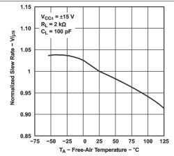
Figure 6-54. Normalized Slew Rate vs Free-Air Temperature
