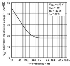
Figure 6-55. Equivalent Input Noise Voltage vs Frequency
