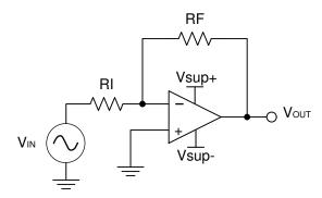
Figure 9-1. Inverting Amplifier
